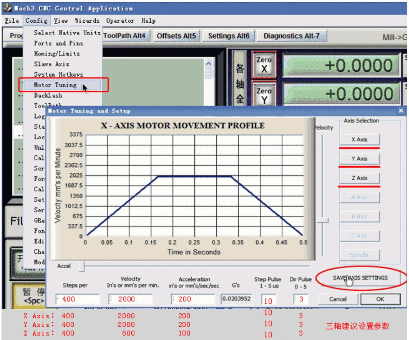
The setup is over, Please close the Mach software that all data setup can be available. And then open it again to check whether all the data is correct otherwise can't run your machine well.
