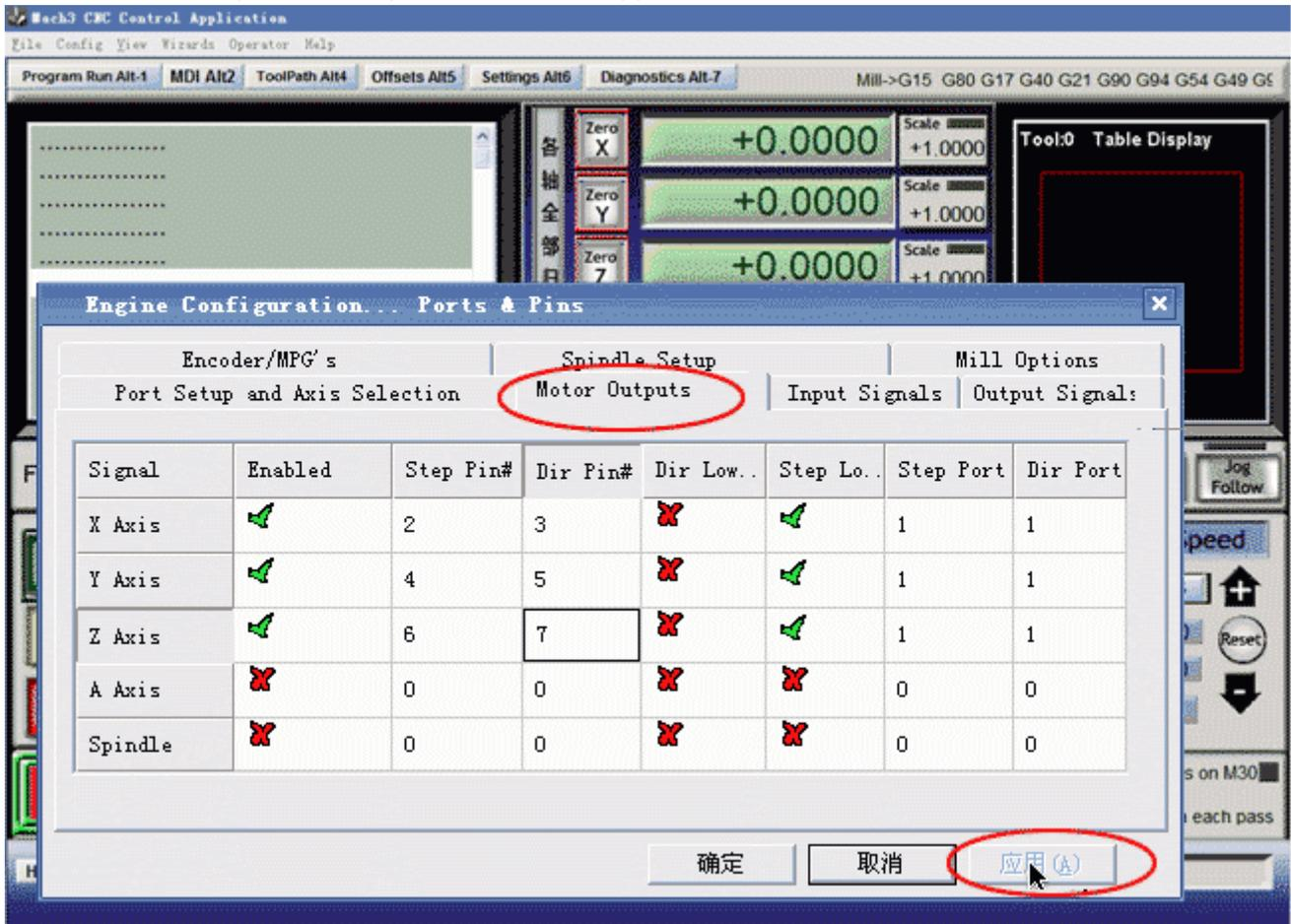
This part is very important, please check your setup is as same as the data above. Even a small error will cause the machine working incorrectly. Do not forget to save the setup.
