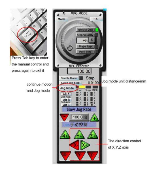
Now the test of the Mach 3 communication with the machine is over. If it still can not realized the manual control, please do as follows:
