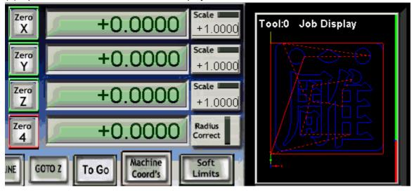
(3)Power on the control box driver, move the spindle tool bit to the left-bottom of the material board by manual control the three axis, the area in the red circle(the image below)is the safe area. The left bottom red-green WCS arrowhead above is the original point, move the spindle bit (without cutter) to this point.
