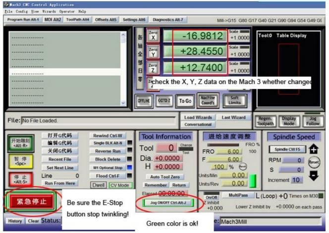
If all the axis can move, please check the direction of the axis coordinate is right(see below).
