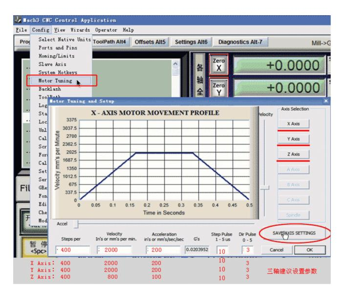
The setup is over, Please close the Mach software that all data setup can be available. And then open it again to check whether all the data is correct otherwise can't run your machine well.
