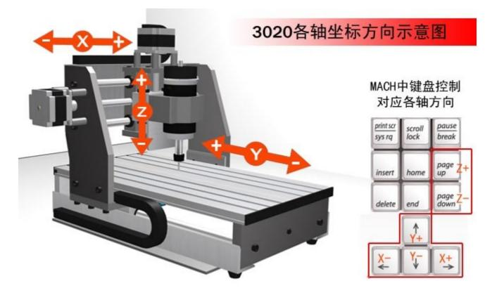
PS: you can use the keyboard to control the direction of the axis, and also you can use the manual control keyboard of Mach 3 by using the mouse to control the movement of the X, Y, Z axis.
