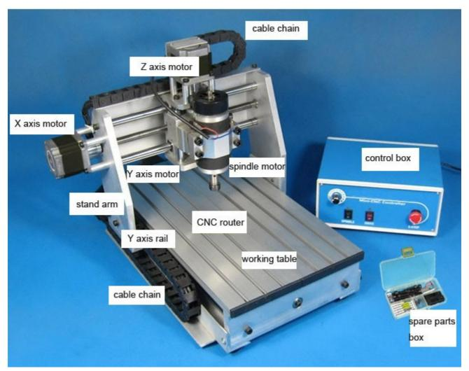
(1) Our machine is made of the aluminum alloy, if you drop it from the top on the floor or hard hit, it will damage the machine. Please put this machine on the stable desk, the thin desk may cause more resonance when it is running.
